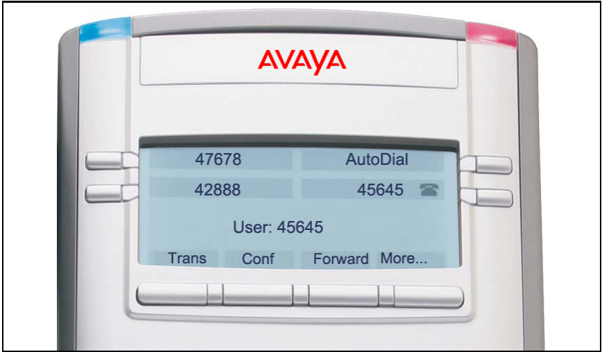
Figure 26: Logged in to an Avaya 1120E IP Deskphone
